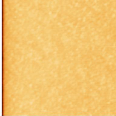
**Fig. 1.** Initial AFM image ( $5\mu\text{m} \times 5\mu\text{m}$ ) of cobalt surface recorded in contact mode (RMS=9.8 Å).
