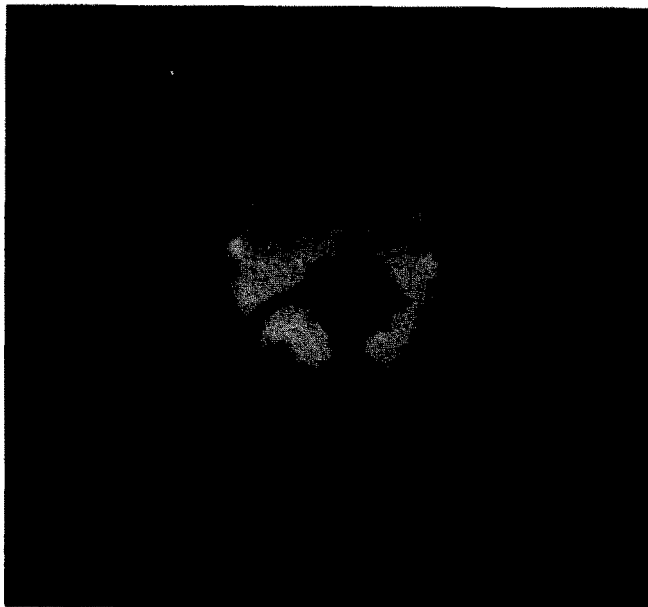
Fig. 2. Diffraction pattern of a xenon monolayer on (100)NaCl at 60 K and 1.1 \times 10^{-6} Torr; the incident energy is 75 eV.
